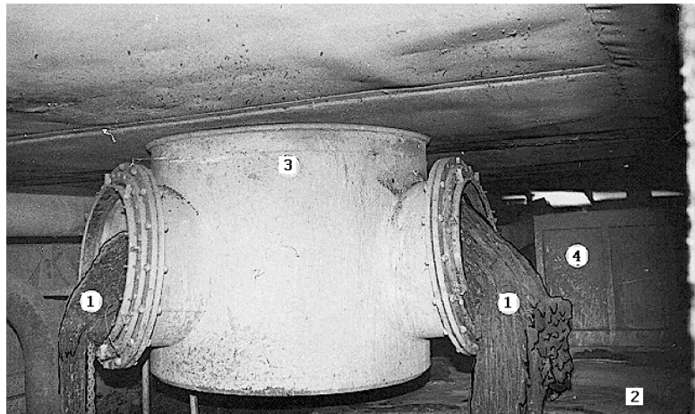
Figure 3-10 - Resolidified molten debris
